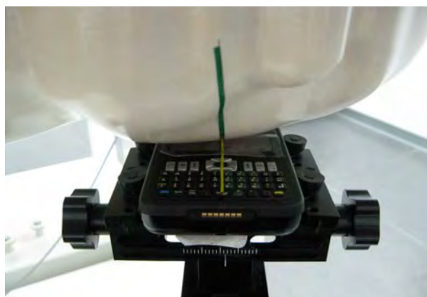
Fig.5 Left Head Section / Cheek-Touch Position
