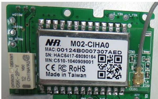
A Stamp Hole installation example of M02 Module with I-PEX Connector
