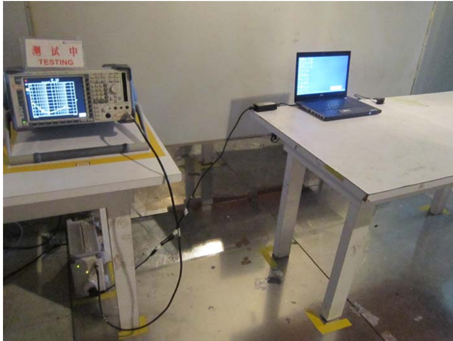
CONDUCTED EMISSION TEST SETUP (FOR CHARGING MODE)
