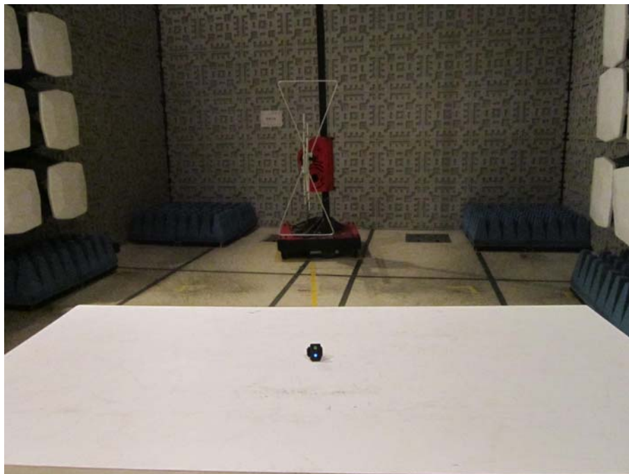
TEST SETUP OF RADIATED EMISSION (30MHz-1GHz)
