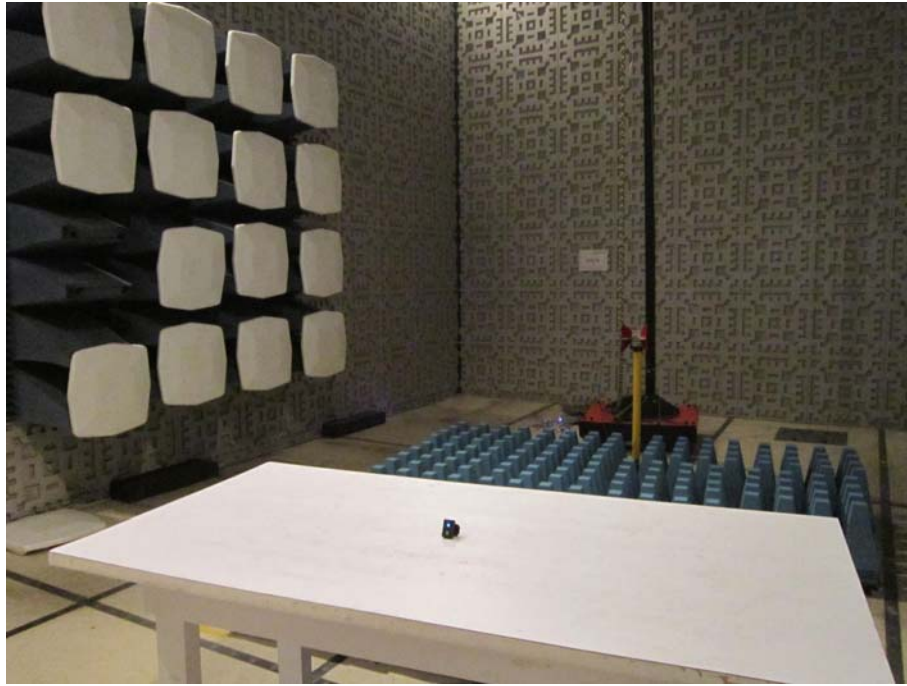
TEST SETUP OF RADIATED EMISSION (above 1GHz)
