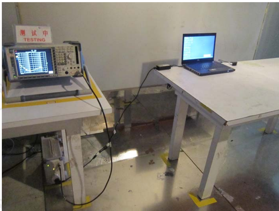
CONDUCTED EMISSION TEST SETUP (FOR CHARGING MODE)
