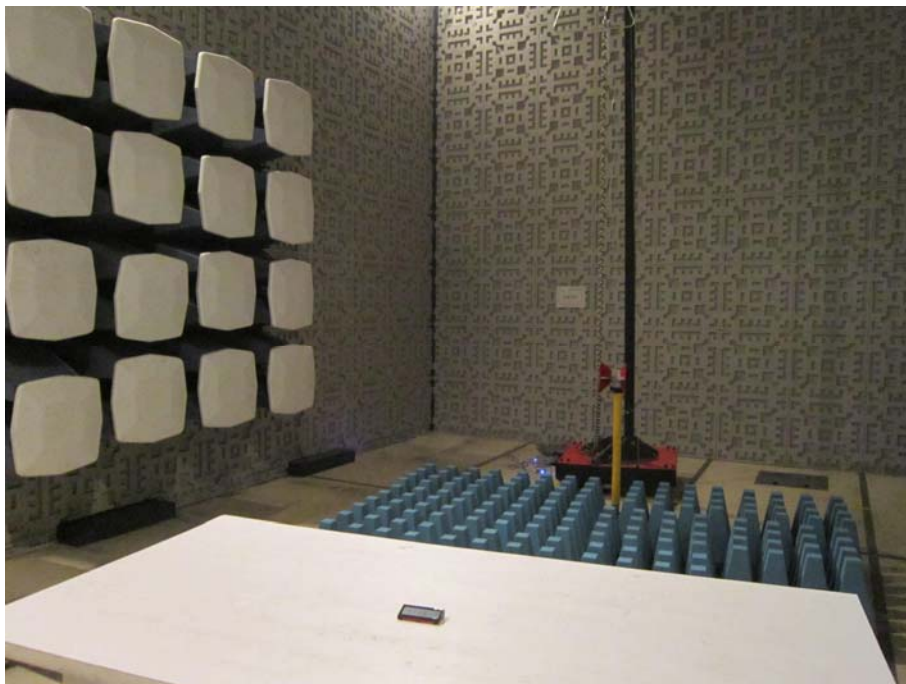
TEST SETUP OF RADIATED EMISSION (above 1GHz)
