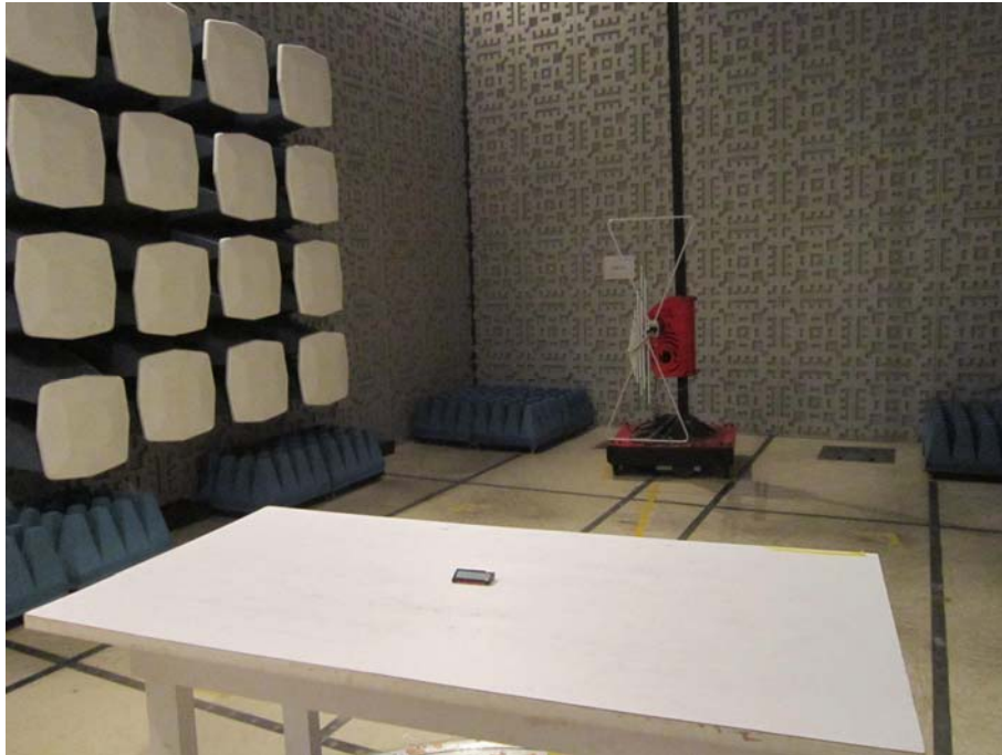
TEST SETUP OF RADIATED EMISSION (30MHz-1GHz)
