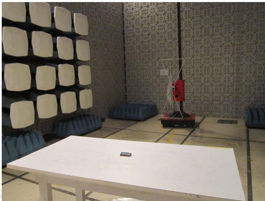
TEST SETUP OF RADIATED EMISSION (30MHZ-1GHZ)
