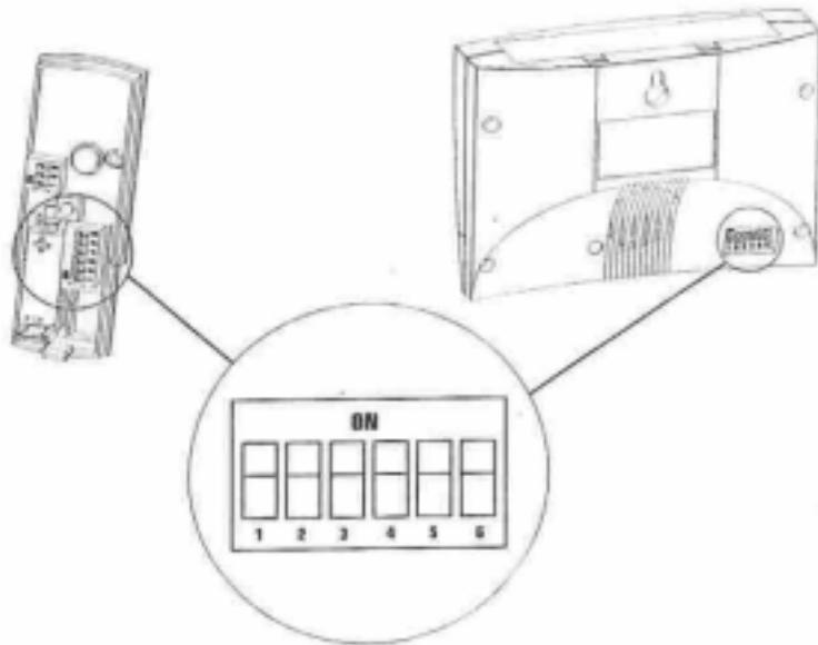
**Important – The position of the code selection switches on the bell push and receiver unit
