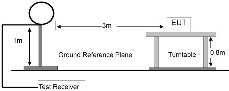
For Radiated Emission 30-1000MHz
