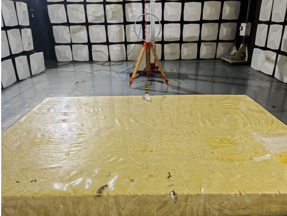
Radiated emission (30-1000MHz)
