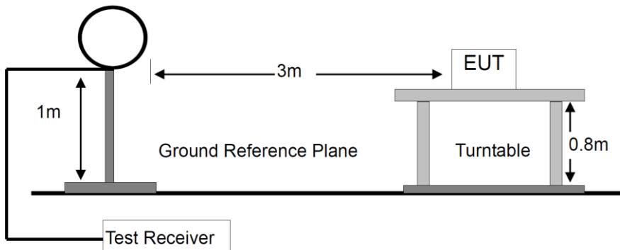
For Radiated Emission 30-1000MHz
