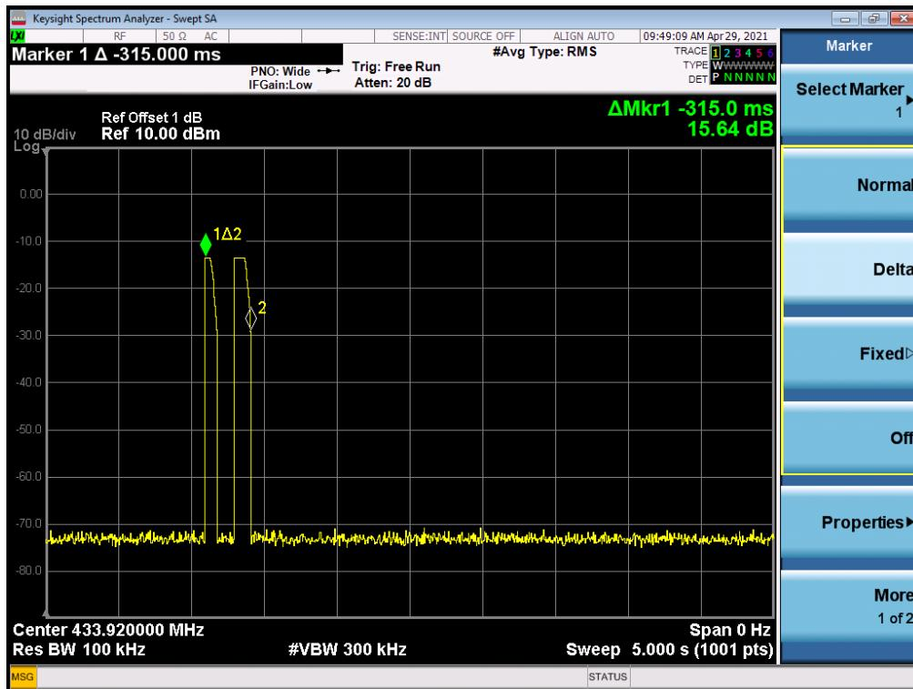
Note: Each transmission contains two long pulses.
