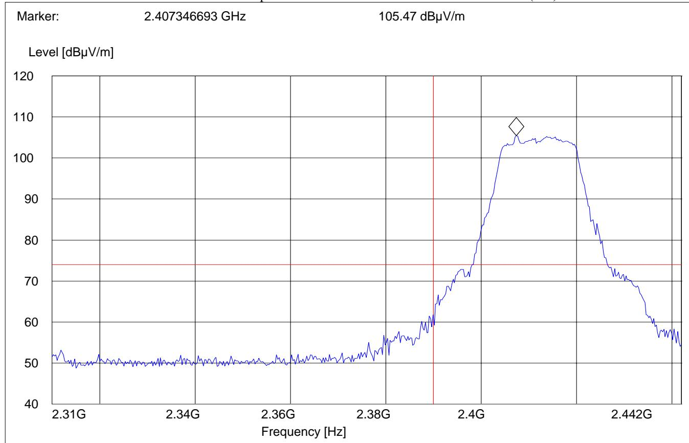
**BAND EDGE COMPLIANCE****§15.247 (c)****High frequency section (spurious in the restricted band 2483.5 – 2500 MHz)****(Average measurement @ 6Mbps)**
