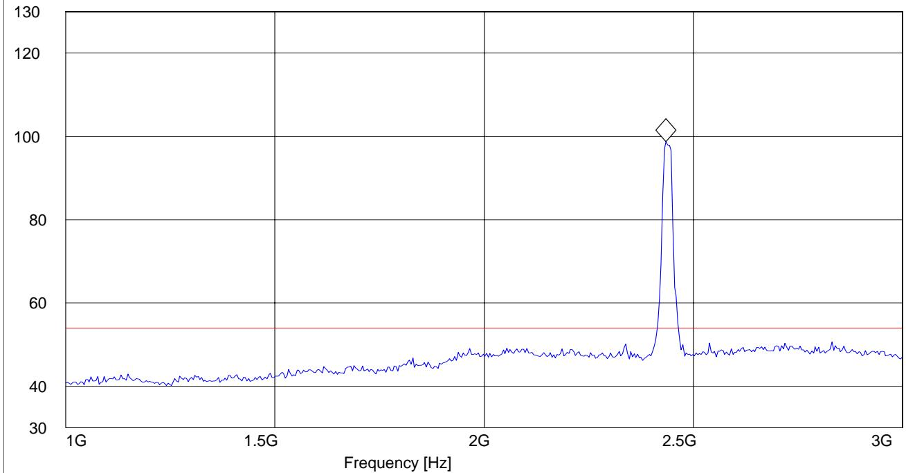
**EMISSION LIMITATIONS - Radiated (Transmitter)****§ 15.247 (c) (1)****Mid Channel (2437MHz): 3GHz – 18GHz****@ 54Mbps (Average measurement)****SWEEP TABLE: "Spuri hi 3-18G"**
