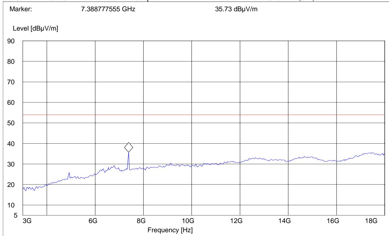
**EMISSION LIMITATIONS - Radiated (Transmitter)** § 15.247 (c) (1)
