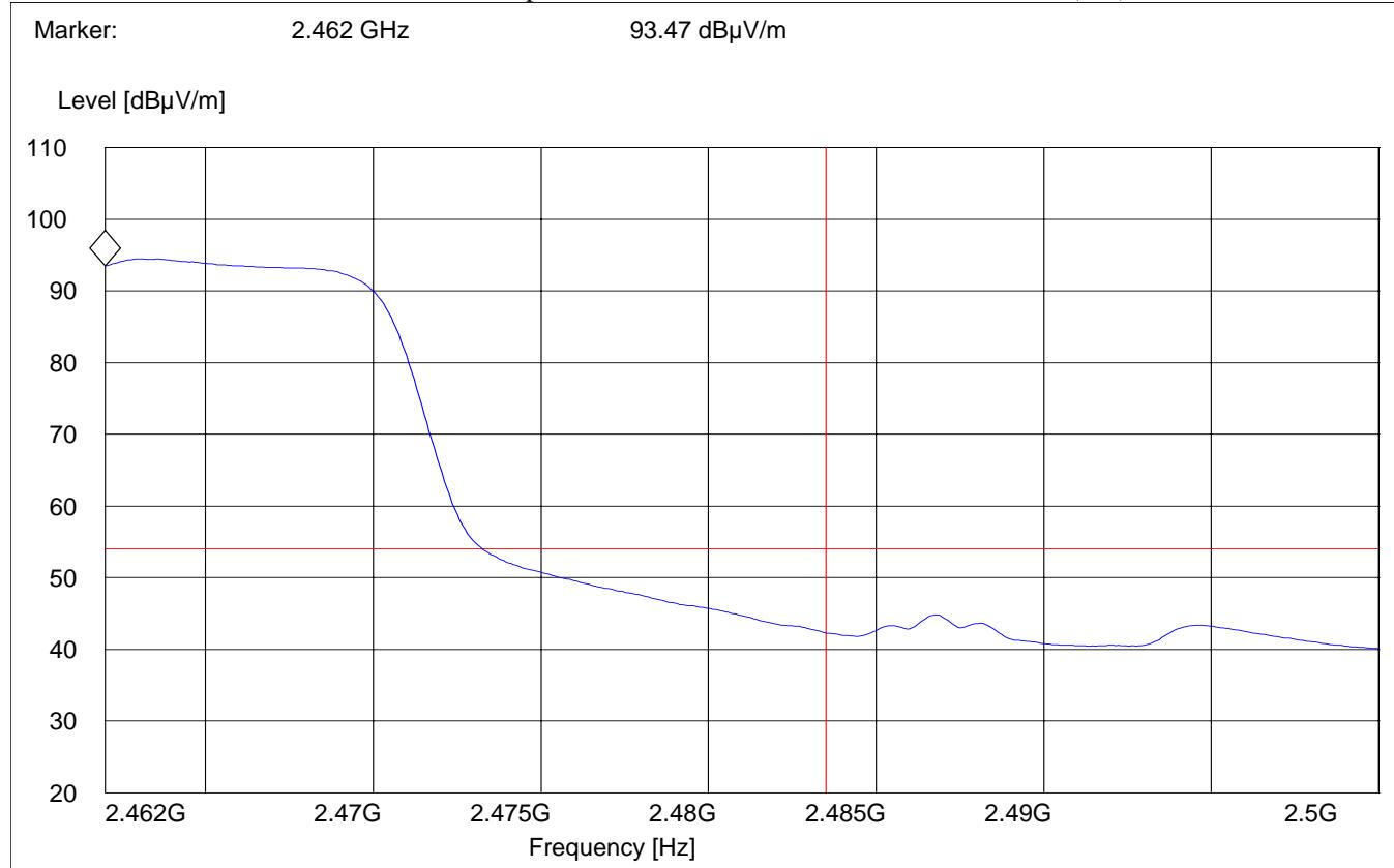
**BAND EDGE COMPLIANCE****§15.247 (c)****High frequency section (spurious in the restricted band 2483.5 – 2500 MHz)****(Peak measurement @ 54Mbps)**
