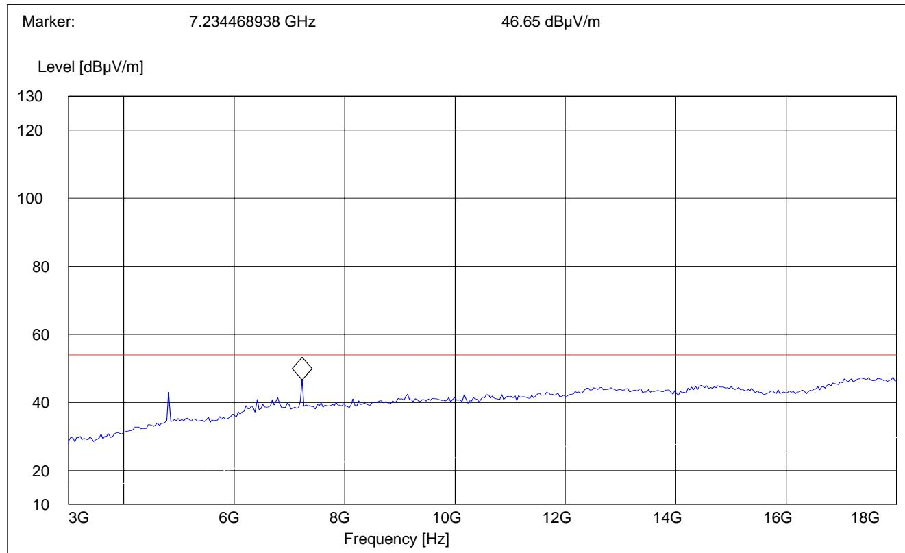
**EMISSION LIMITATIONS - Radiated (Transmitter)****§ 15.247 (c) (1)****Mid Channel (2437MHz): 1GHz – 3GHz****@ 54Mbps****Note: The peak above the limit line is the carrier freq.****SWEEP TABLE: "Spuri hi 1-3G"**
