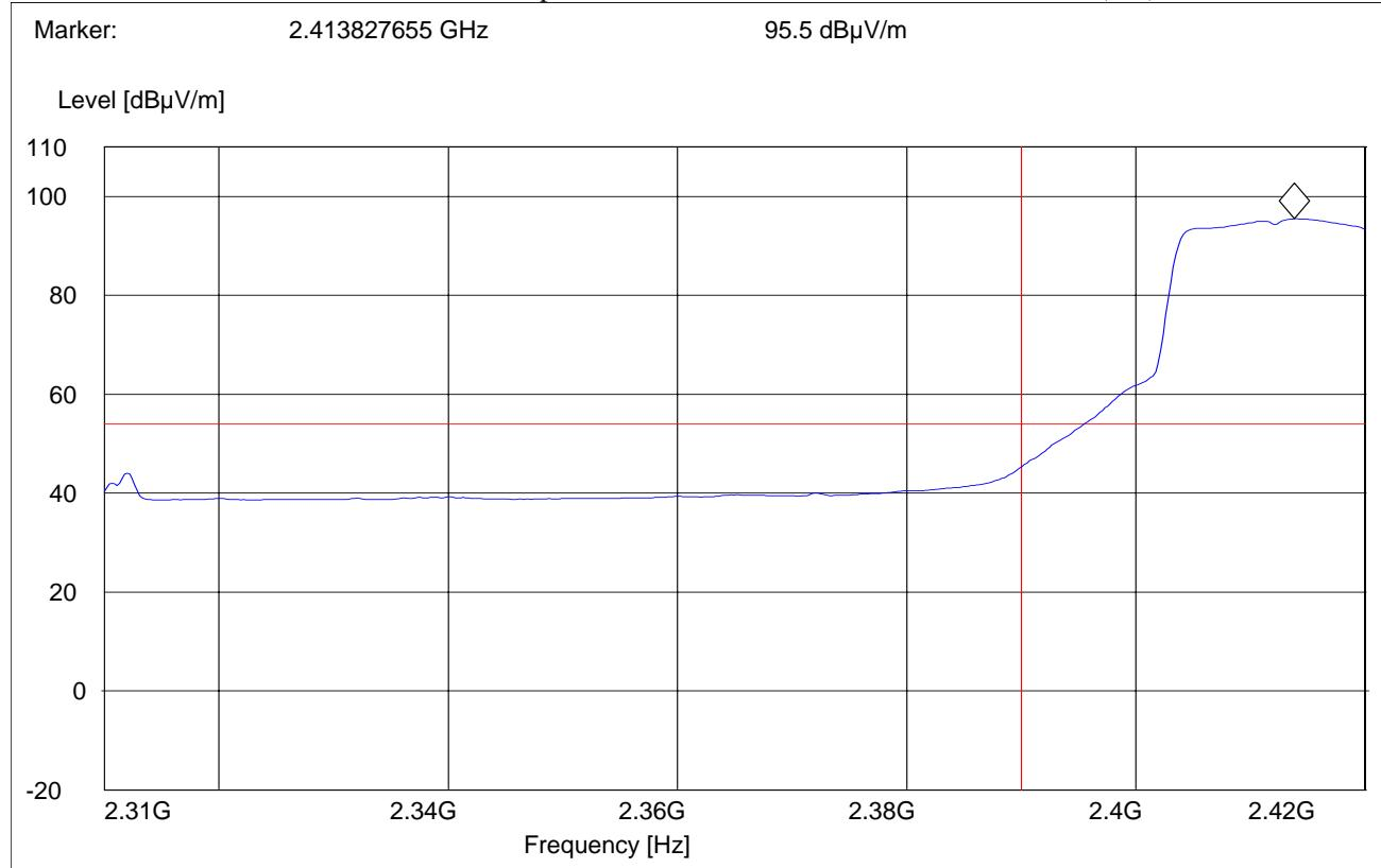
**BAND EDGE COMPLIANCE****§15.247 (c)****Low frequency section (spurious in the restricted band 2310 – 2390 MHz)****(Peak measurement @ 54Mbps)**
