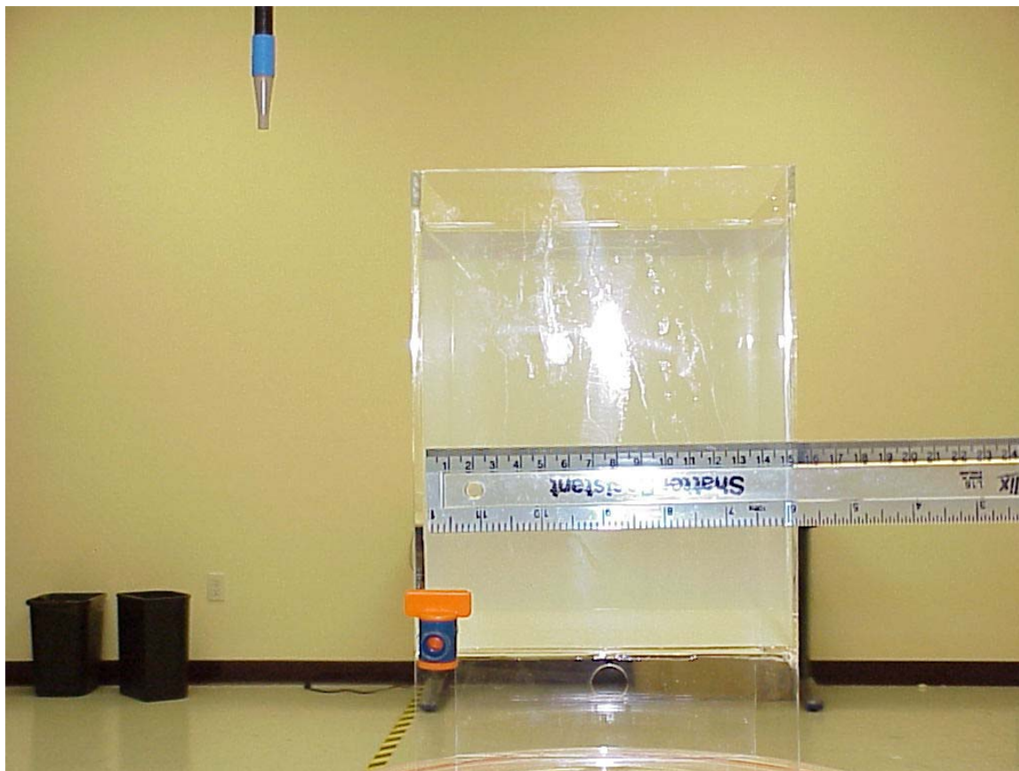
Photo 5 Photo to demonstrate 15 cm Z-axis flat phantom
