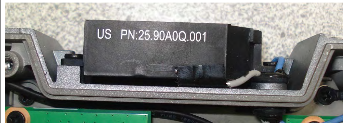
WLAN AUX (CHAIN B) TRANSMIT DIVERSITY ANTENNA HOUSING
