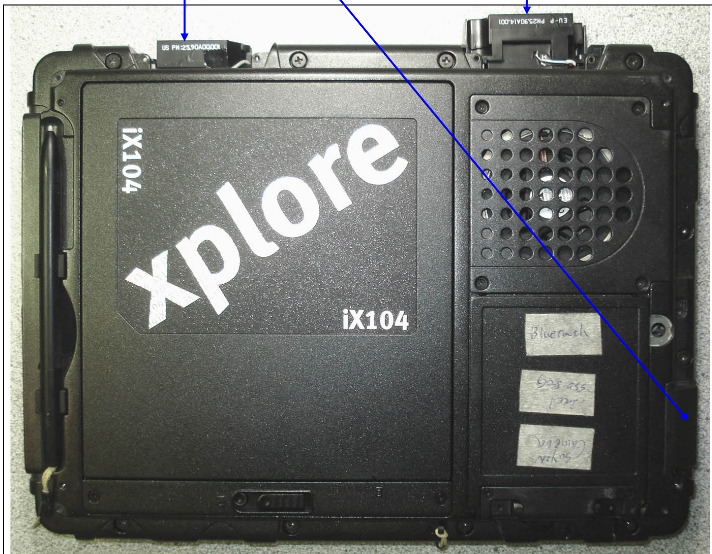
ANTENNA LOCATION(S) - BOTTOM SIDE OF iX104C5 TABLET PC (with "Pump-Up" WWAN Antenna)
