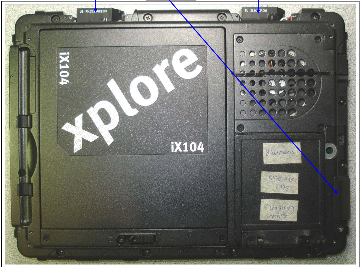
WLAN & BLUETOOTH ANTENNA LOCATIONS – BOTTOM SIDE OF ix104C5 TABLET PC
