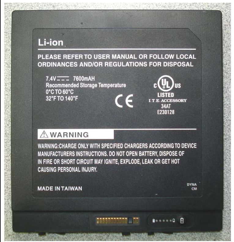
Back Side of Li-ion Battery
