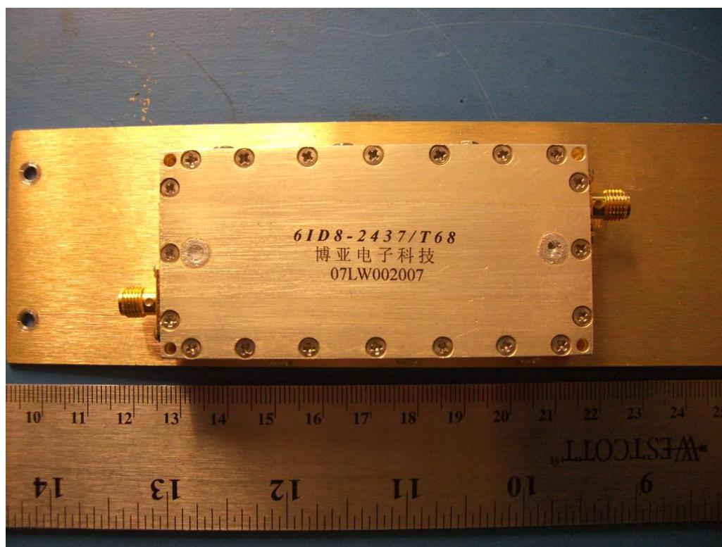
**15.23 Filter with Cover off - Front View**
