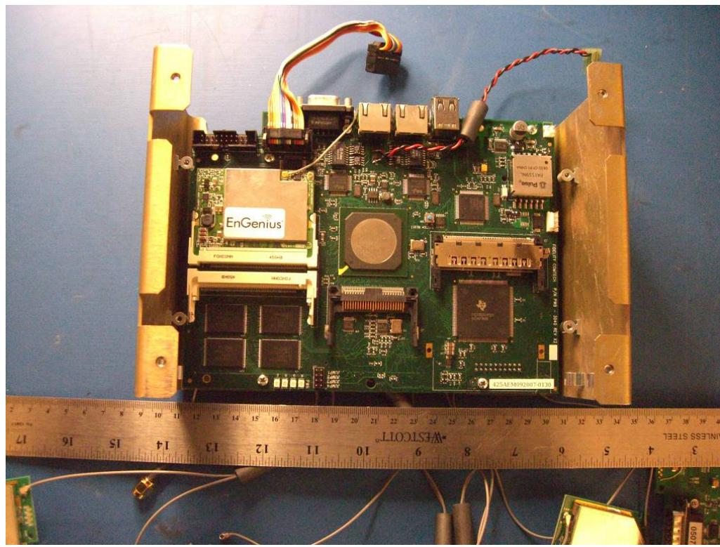
**15.15 Main PCB Board with Radio Components View**
