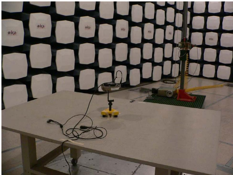
**7.7 Conducted Emissions Front View (Murata Antenna)**
