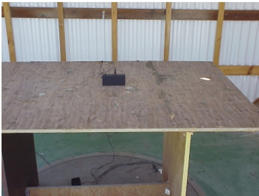
Photo #2 Radiated emission test setup
