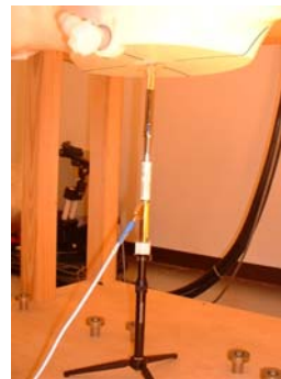
2450MHz System performance check setup
