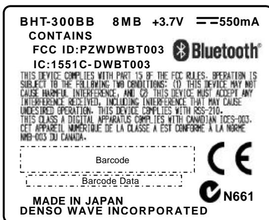
Fig. Label Layout of Scanner Assy
