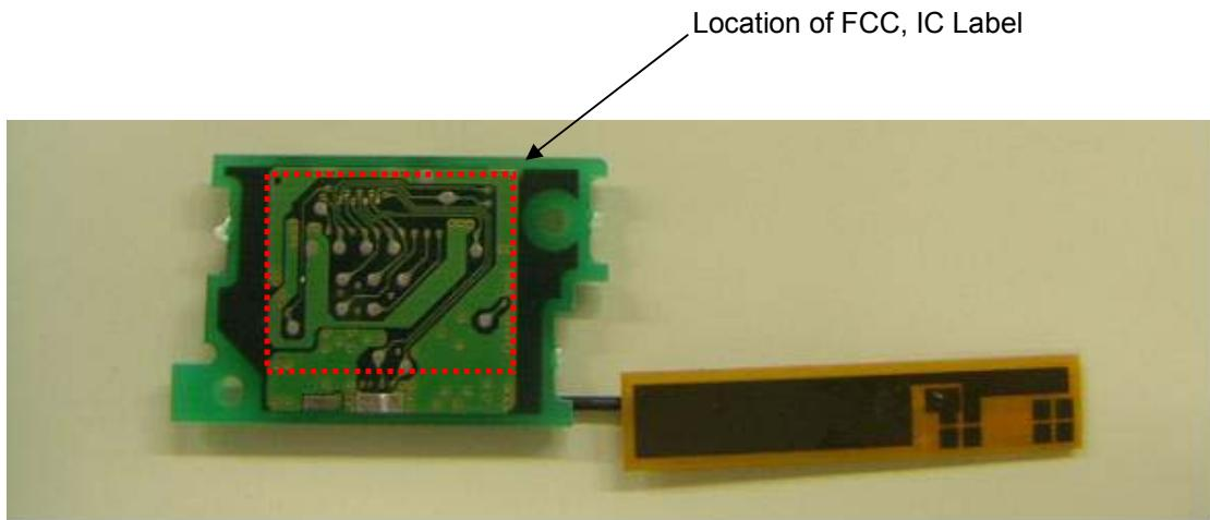
**Fig. Photo of Bluetooth Board (Solder side)**
