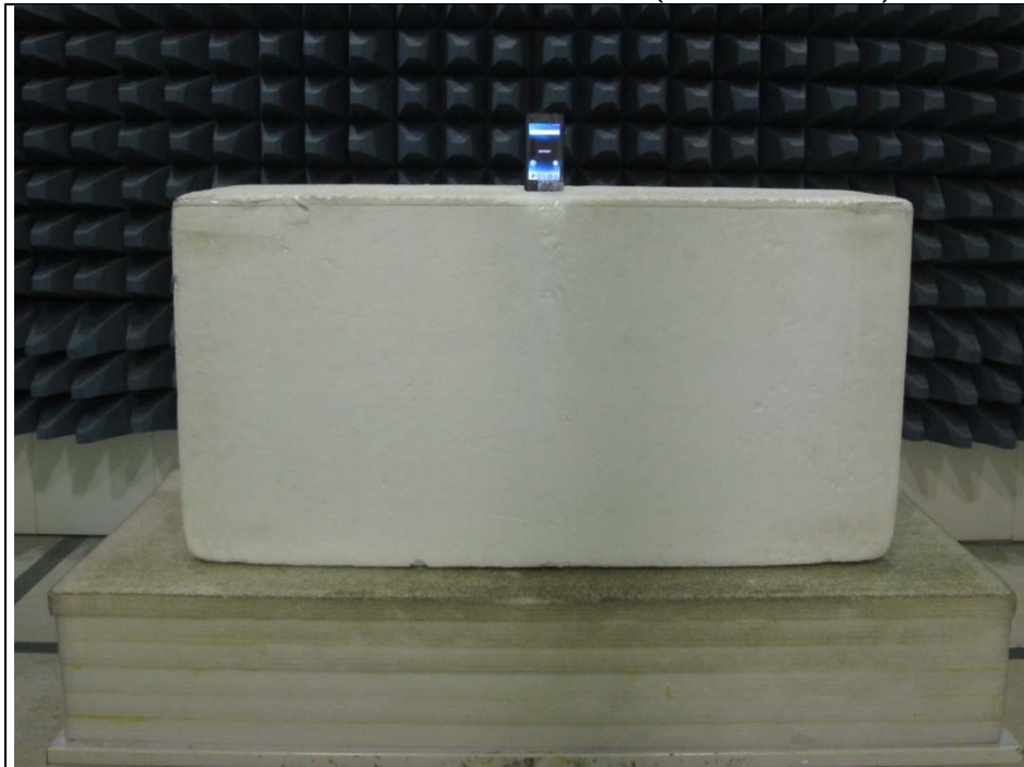
Radiated Emissions above 1 GHz Test (For WLAN 5GHz)
