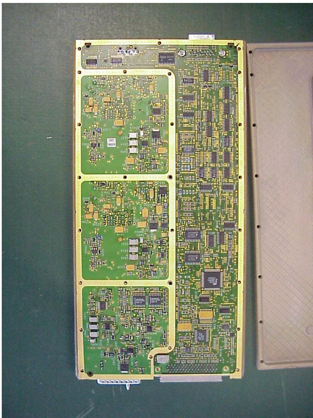
**Photographs of the equipment, Modulator and frequency synthesis card**
