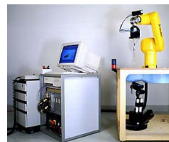
Fig. 1 SAR Test Setup
