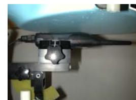
Figure 24. Mouth SAR Test Setup
