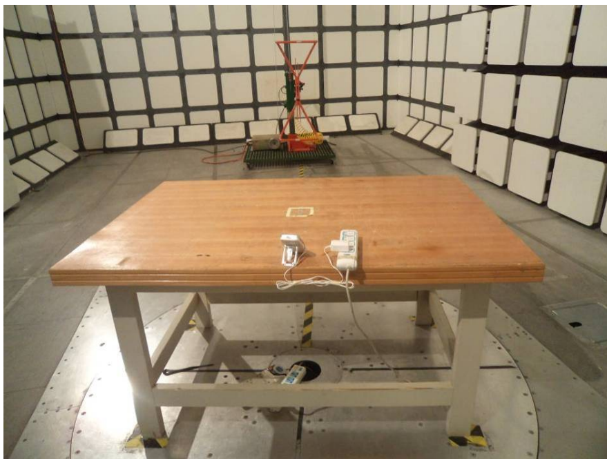
Radiated Emissions – Rear View (30-1000 MHz)
