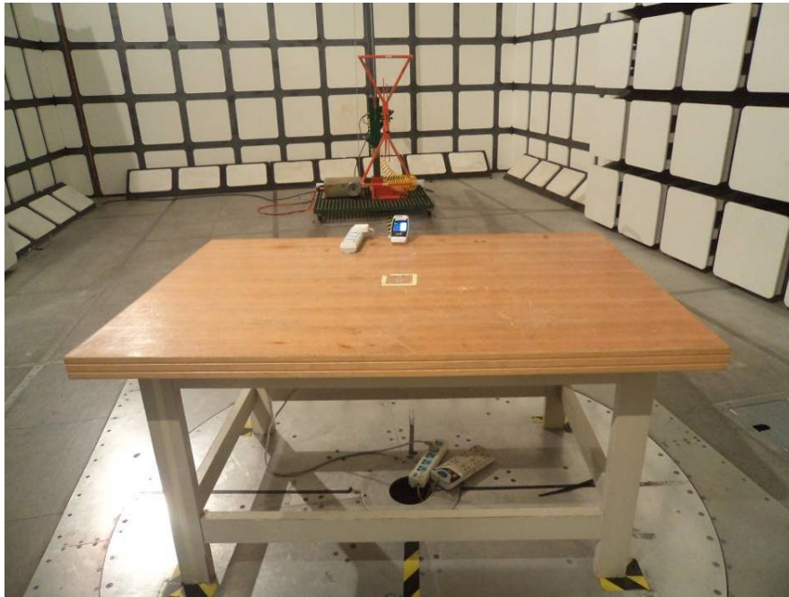
Radiated Emissions – Front View (30-1000 MHz)
