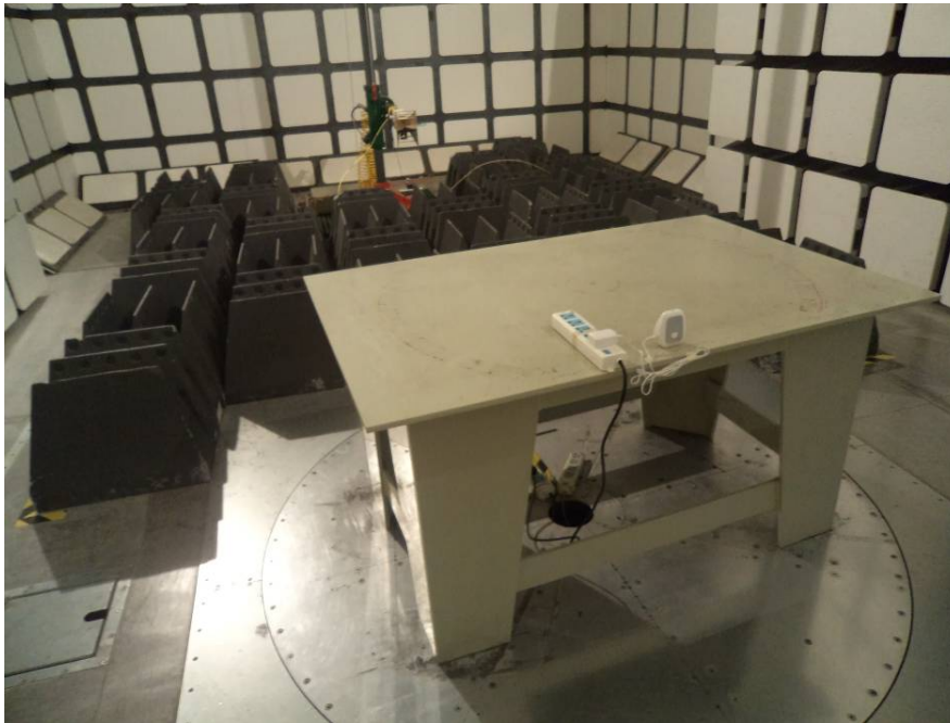
Radiated Emissions – Front View (1-25 GHz)
