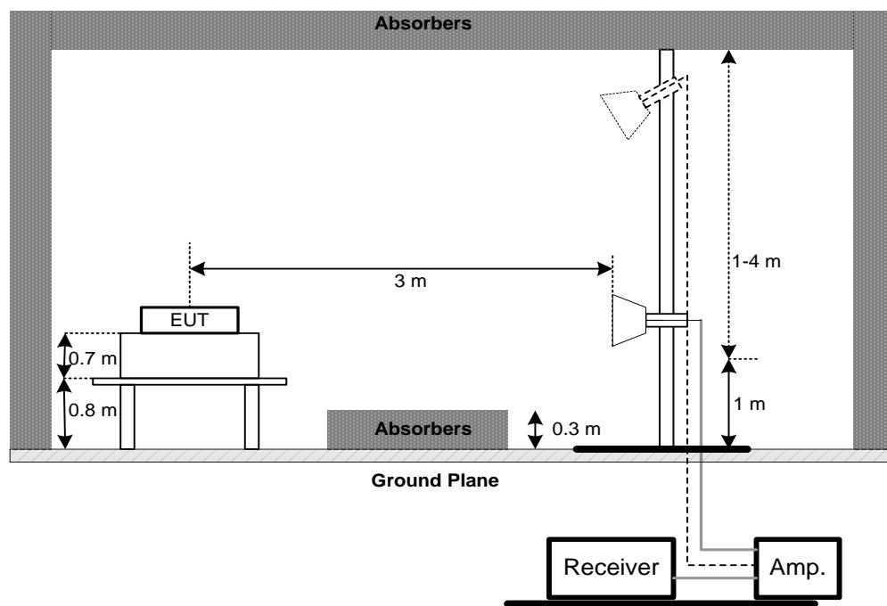
(C) For radiated emissions below 30MHz
