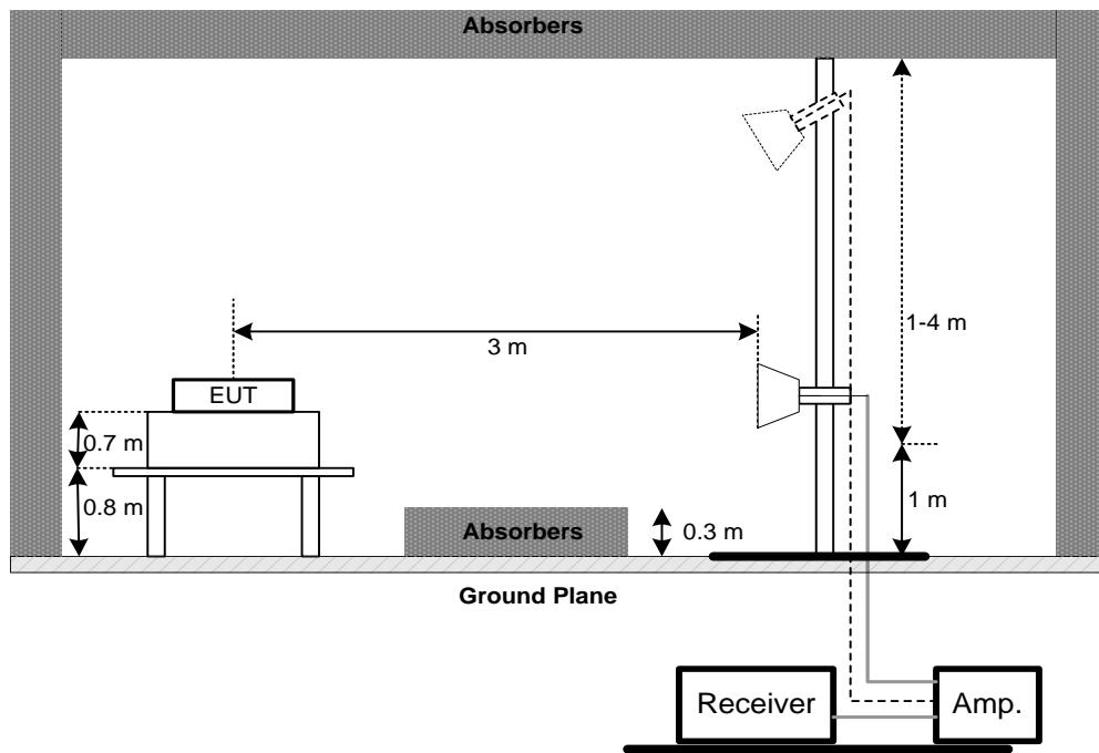
(C) For radiated emissions below 30MHz
