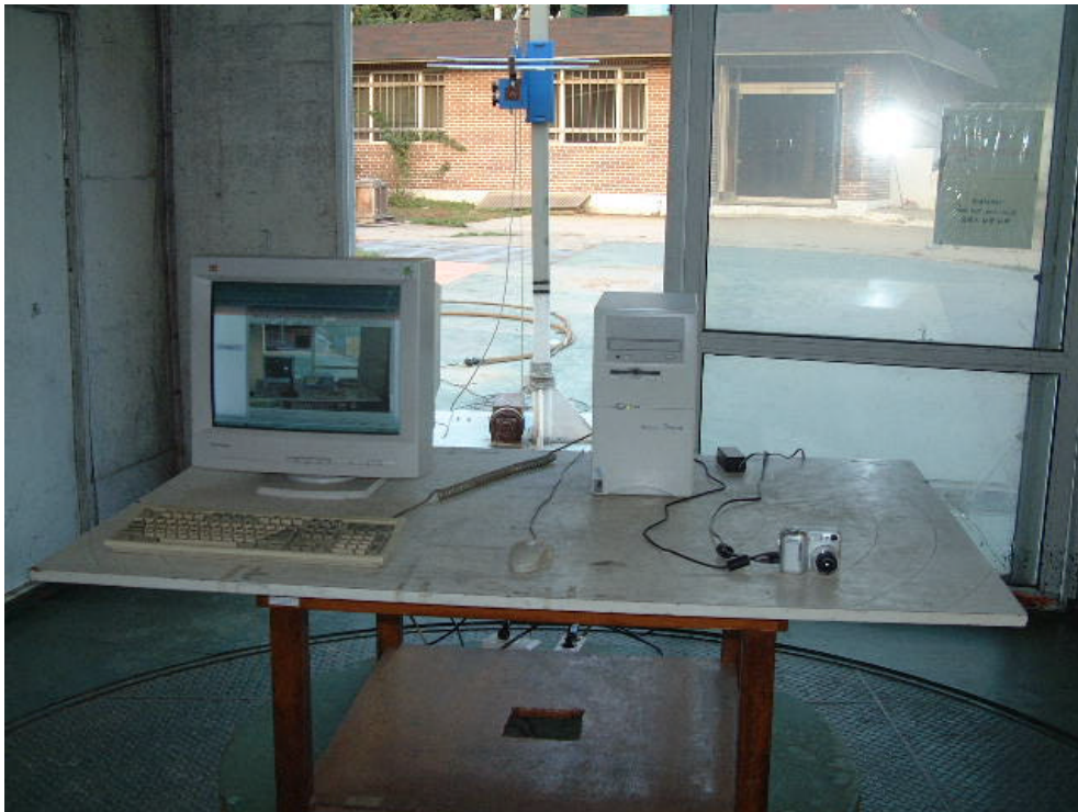
RADIATED EMISSION SETUP PHOTOGRAPH - FRONT VIEW ( 300- 1000 MHz )
