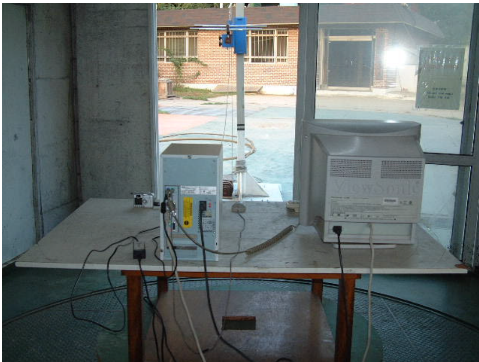
RADIATED EMISSION SETUP PHOTOGRAPH - REAR VIEW ( 300 - 1000 MHz )
