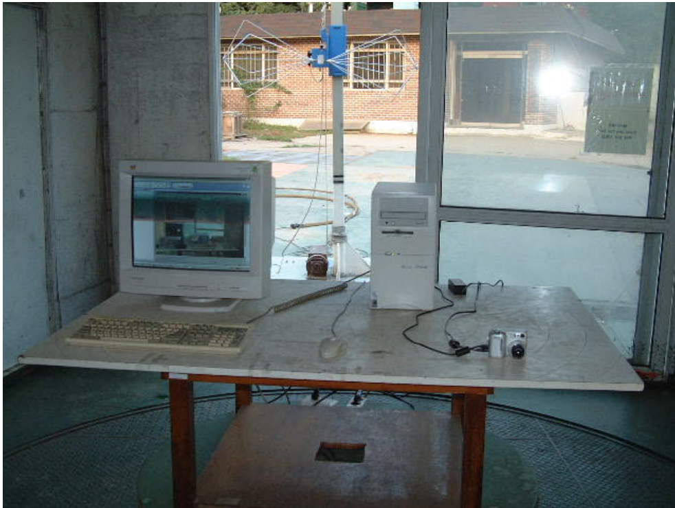
RADIATED EMISSION SETUP PHOTOGRAPH - FRONT VIEW ( 30 - 300 MHz )
