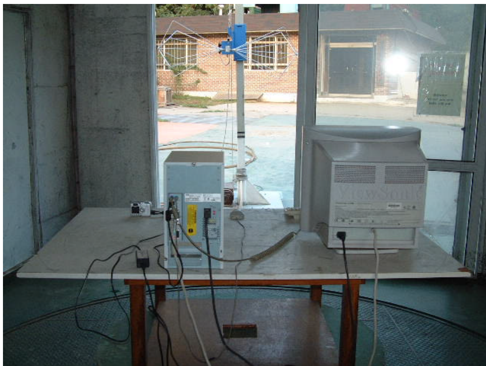
RADIATED EMISSION SETUP PHOTOGRAPH - REAR VIEW ( 30 - 300 MHz )
