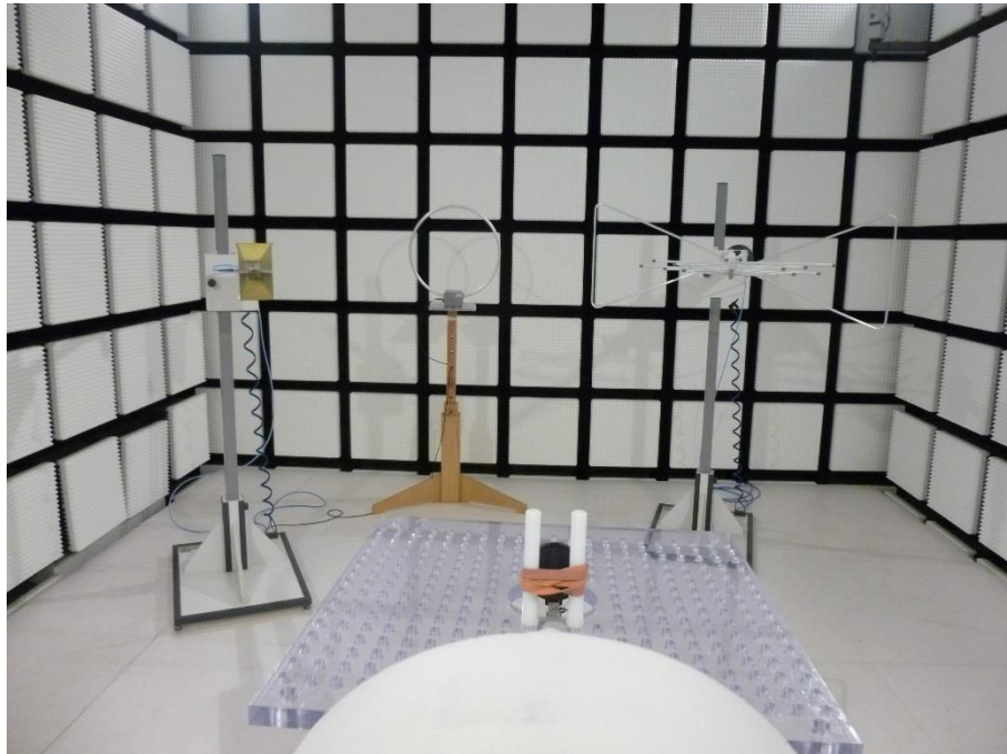
Photo 4 (RSE Setup 9 kHz to 30 MHz & 1 GHz to 12.75 GHz):
