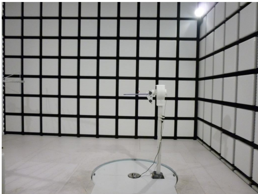
Photo 2 (RSE Setup 9 kHz to 30 MHz & 1 GHz to 12.75 GHz):
