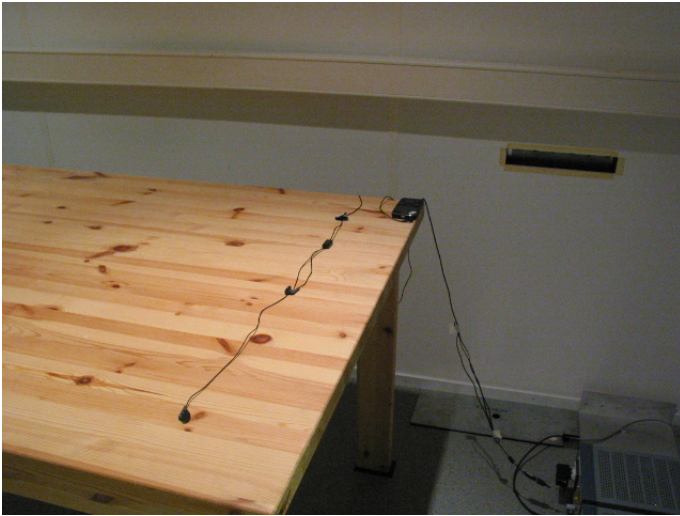
Picture 3 AC powerline conducted emission measurement 15C
