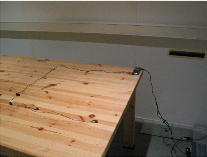
Picture 3 AC powerline conducted emission measurement 15C
