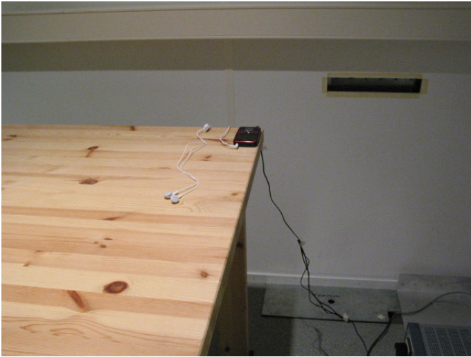
Picture 3 AC powerline conducted emission measurement 15C
