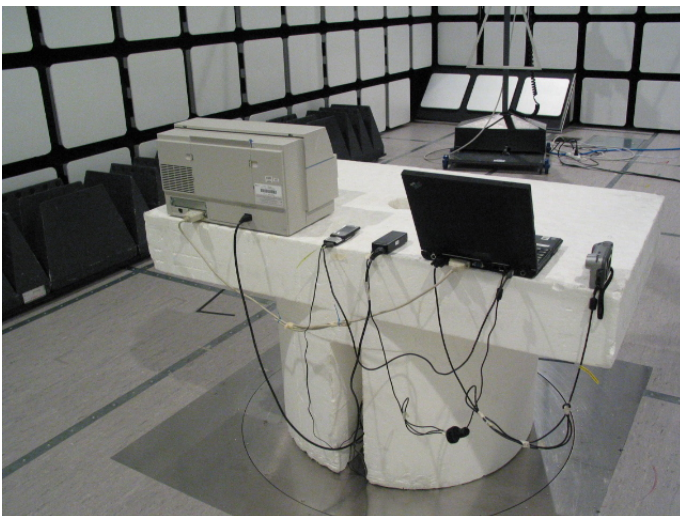
Picture 2 Radiated emission measurement GSM RX/BT TX/WLAN TX + Computer peripherals
