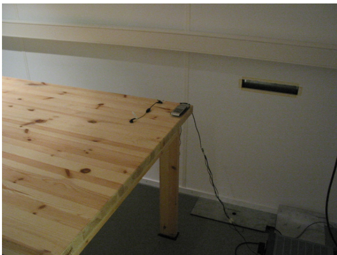
Picture 3 AC powerline conducted emission measurement BT TX/WLAN TX
