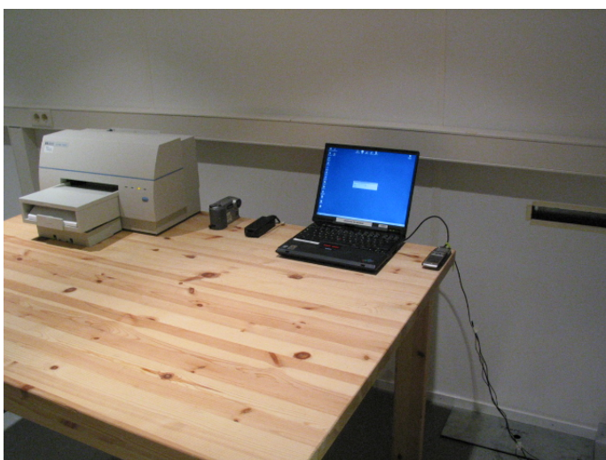
Picture 4 AC powerline conducted emission measurement GSM RX/BT TX/WLAN TX + Computer peripherals
