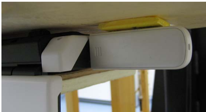
Device directly connected to a USP port of the laptop computer, side 4 facing the phantom. The 0.5 cm spacer was removed before the test.
