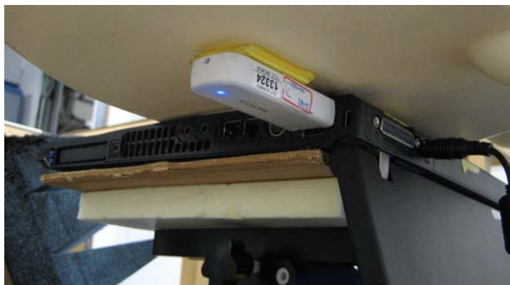
Device directly connected to a USP port of the laptop computer, side 1 facing the phantom. The 0.5 cm spacer was removed before the test.
