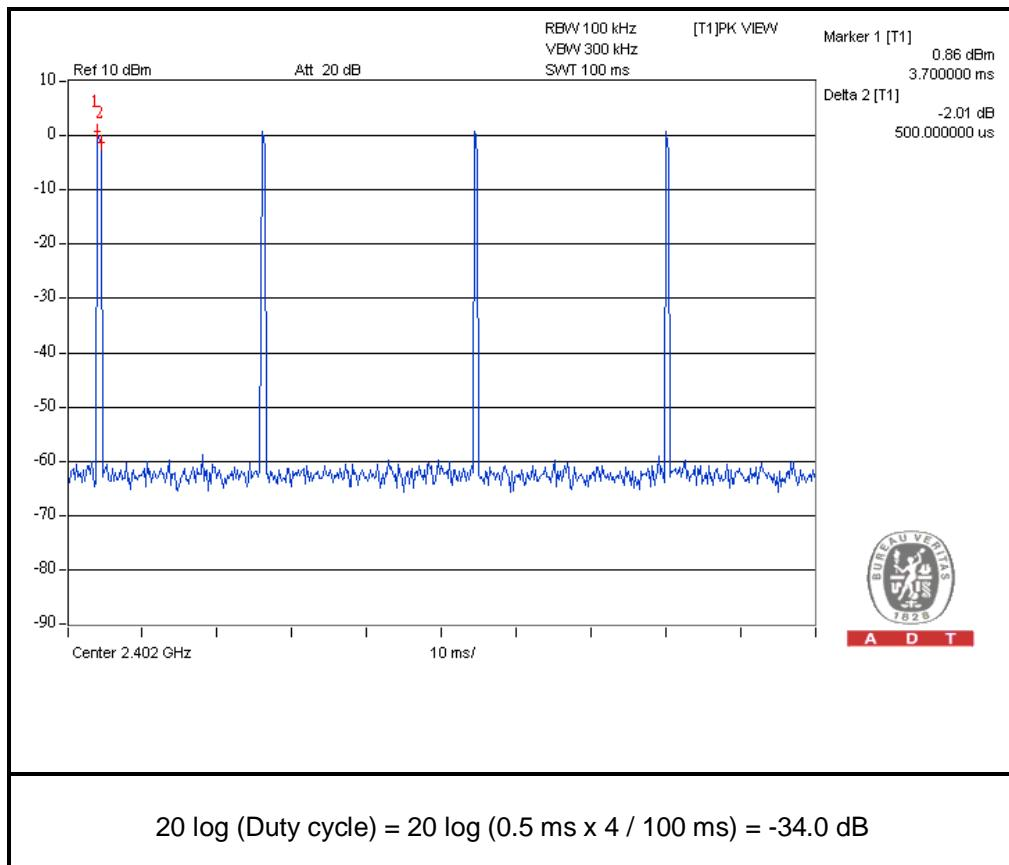
$$20 \log (\text{Duty cycle}) = 20 \log (0.5 \text{ ms} \times 4 / 100 \text{ ms}) = -34.0 \text{ dB}$$
