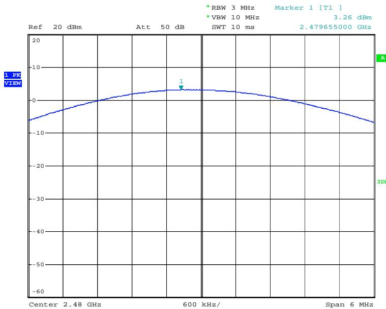
Modulation Type:  $\pi/4$  –DQPSK
