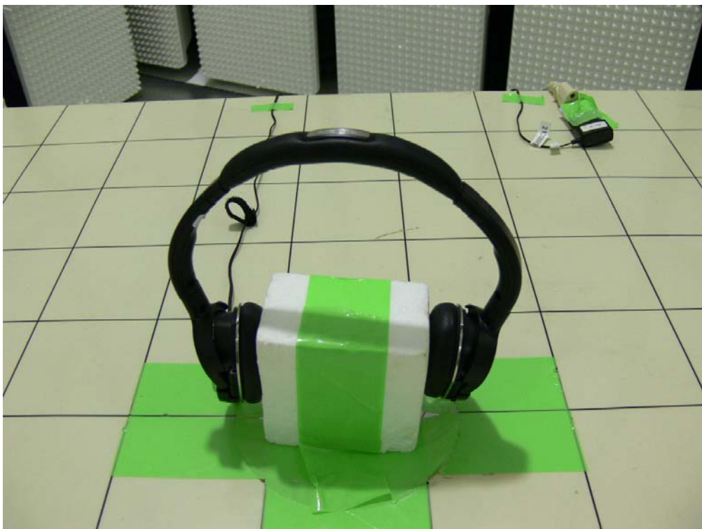
Photograph 3: Set-up for Radiated Emission, EUT Configuration Z-Axis
