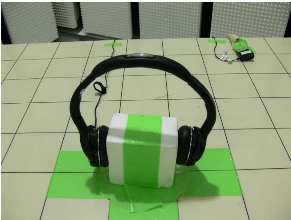
Photograph 3: Set-up for Radiated Emission, EUT Configuration Z-Axis
