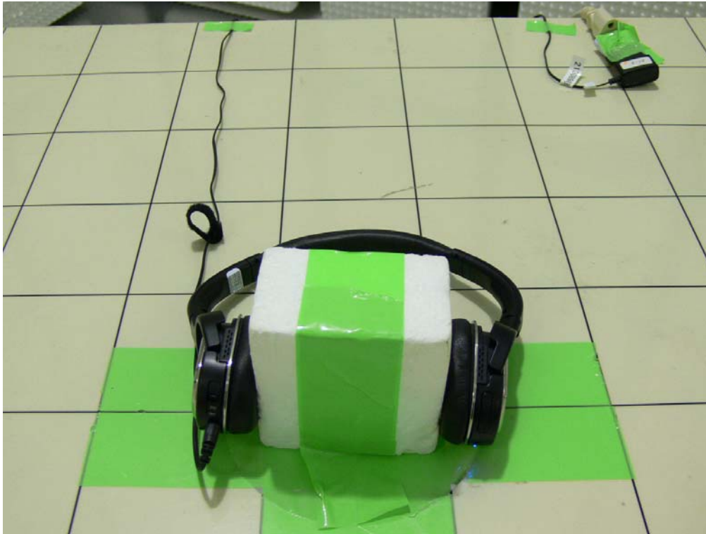
Photograph 2: Set-up for Radiated Emission, EUT Configuration X-Axis
