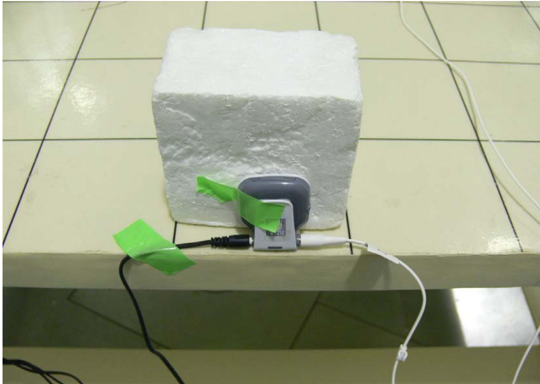
Photograph 4: Set-up for Radiated Emission, EUT Configuration Z-Axis
