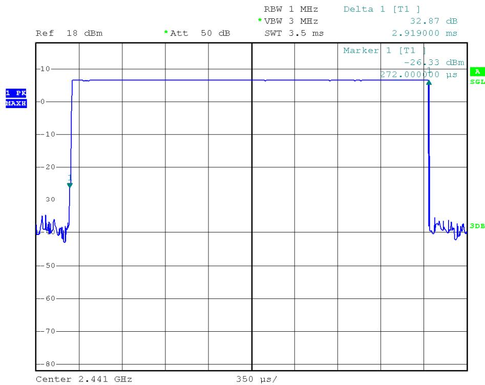
Modulation Type:  $\pi/4$  –DQPSK
