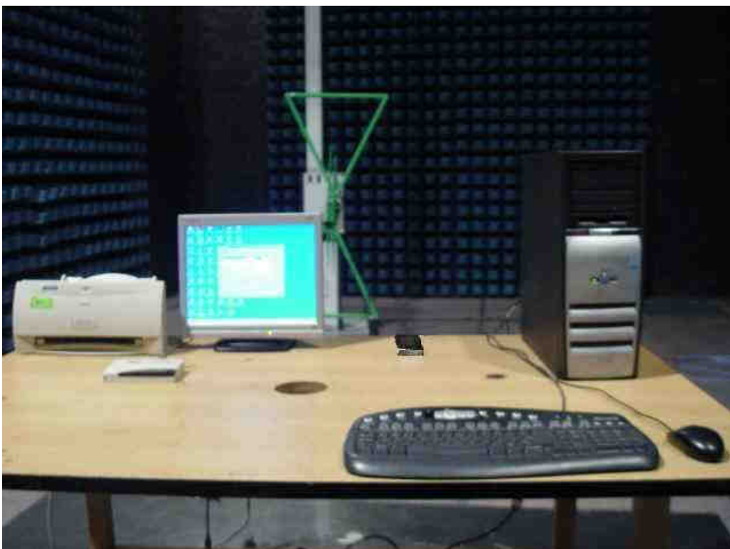
Photograph 2: Set-up for Radiated Emissions
