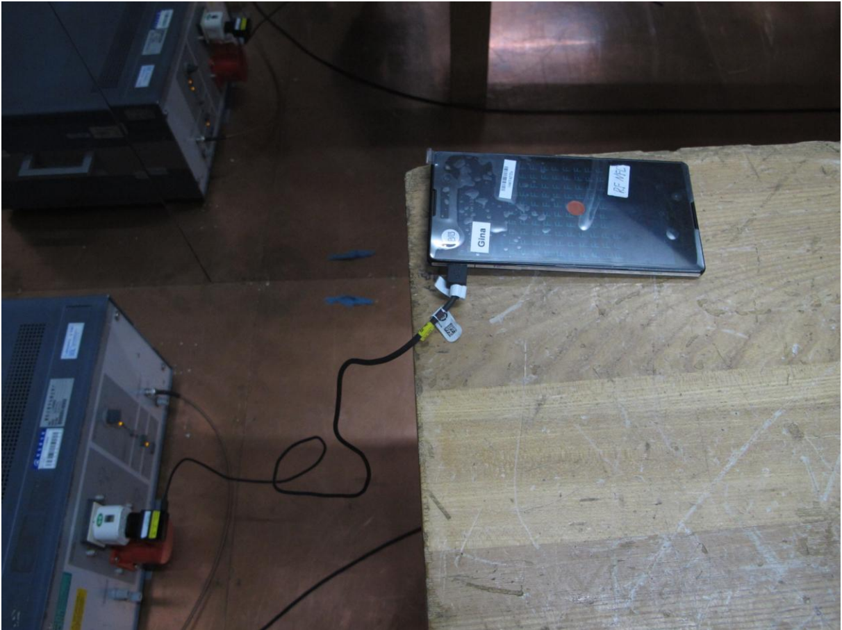
Picture C-3: Conducted Emissions Measurements
