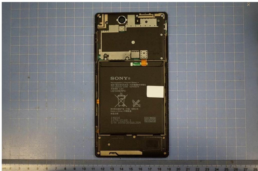
Mobile Phone Disassembly and Inbuilt Battery
