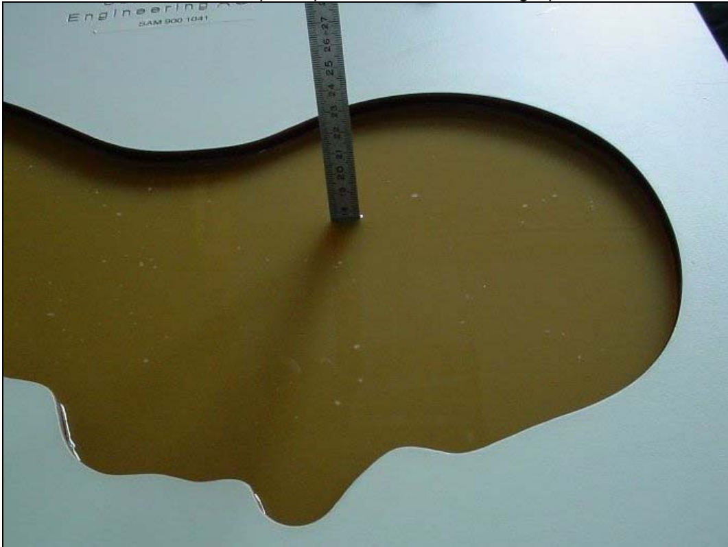
Photo 12: Liquid depth 5 GHz body simulating liquid
