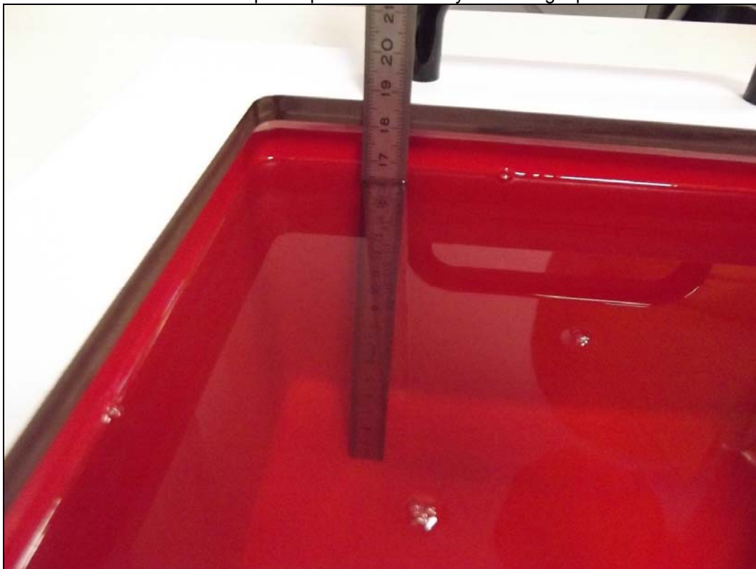
Photo 2: Liquid depth 750 MHz body simulating liquid
