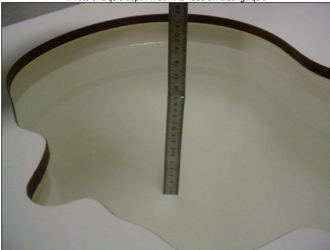
Photo 6: Liquid depth 1750 MHz body simulating liquid
