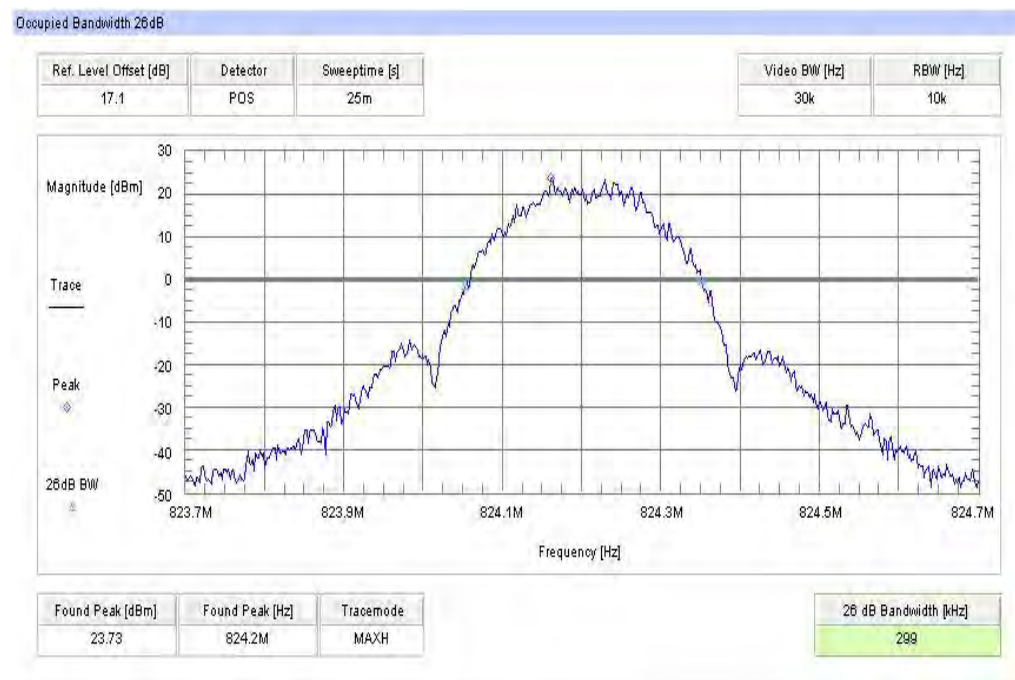
Plot 8: Channel 128 (-26 dBc BW) - 8-PSK
