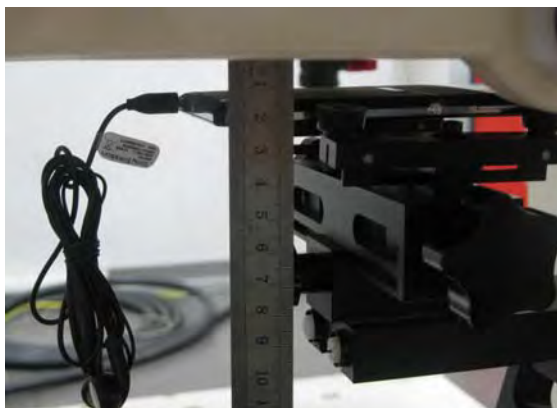
Fig.10 EUT back side with headset (MH410C) to flat phantom
