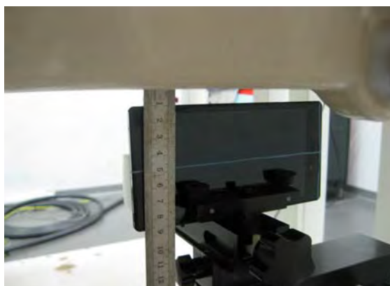
Fig.16 EUT left to flat phantom
