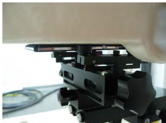
Fig.18 EUT back to flat phantom
