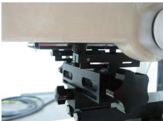
Fig.17 EUT front to flat phantom
