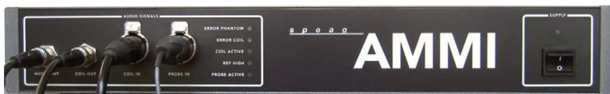
Fig. 5.3 AMMI front panel
