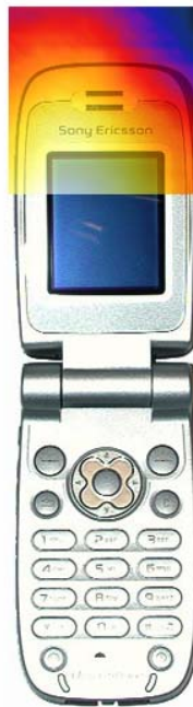
Figure 28 Sample H-field Scan Overlay
