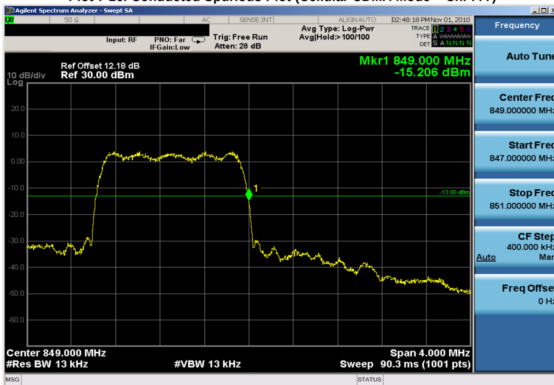
Plot 7-20. Band Edge Plot (Cellular CDMA Mode – Ch. 777)
