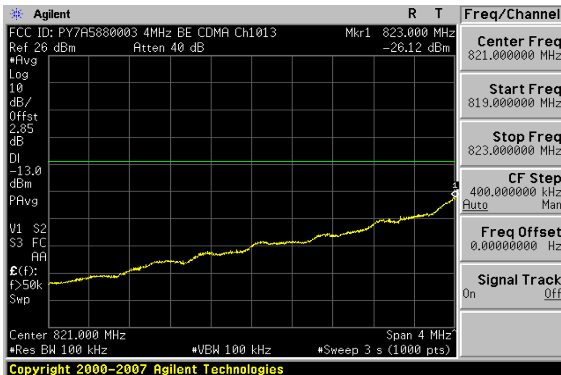
Plot 7-4. 4MHz Span Plot (Cellular CDMA Mode – Ch. 1013)
